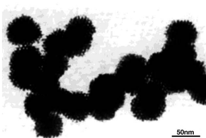
Figure 1.15 TEM image of Pt nanoparticles that have been produced by lyotropic liquid crystal templating. Porous structures can be seen and are spaced in an hexagonal array. (Reprinted with permission from Ref. [54]. ©1997 Wiley-VCH Verlag GmbH & Co. KGaA.)
